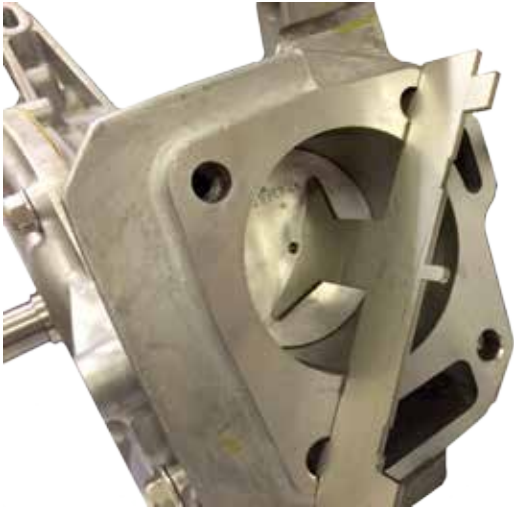
With the piston at BDC, this gauge must sit flush on the deck face
