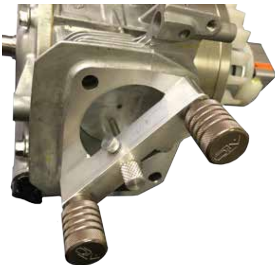
Using the bridge tool as a piston stop when determining ignition timing
