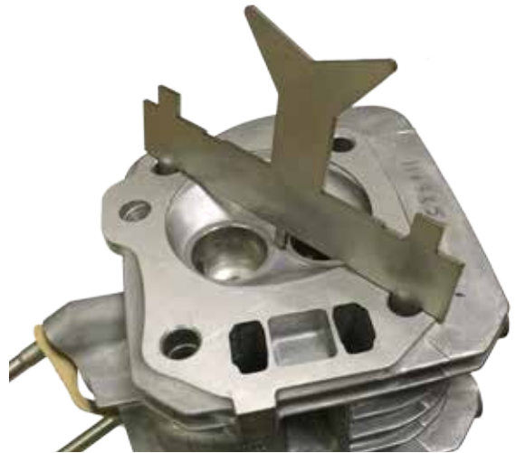
With the lug sitting above the land between the valves, this gauge must sit flush on the cylinder head face. n.b. this gauge is for T2 head only
