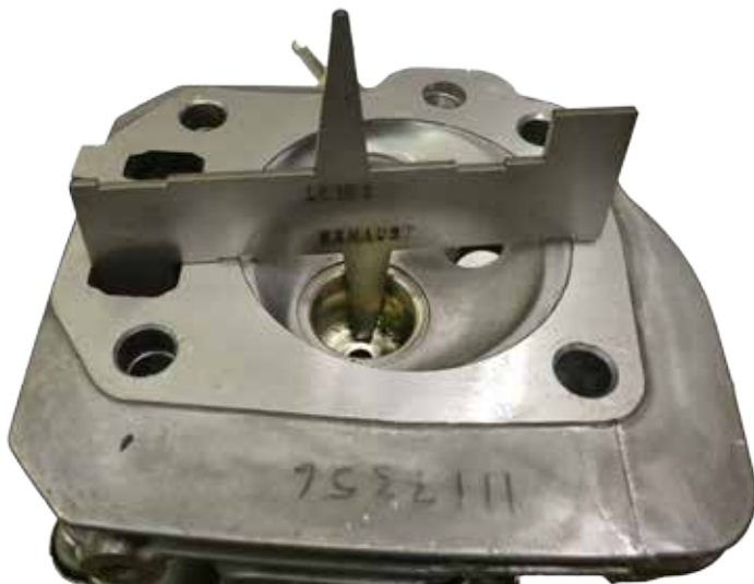
With the lug sitting on the land around the valve guide, this gauge must NOT sit flush on the cylinder head face, but rock
